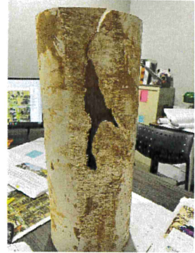
Figure 1 - Water line damaged during work done in the right of way.
